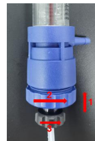
Figure 3.2 Installation of Bottom plungers
